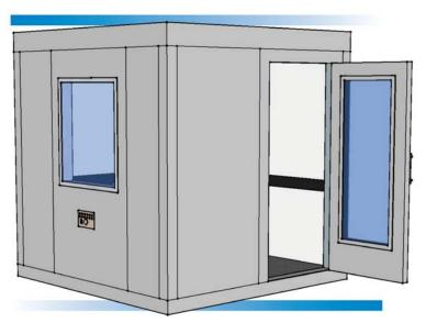
The 40a Classic Series Single-Wall (individual room) construction is a single or multiple occupancy room constructed of four inch thick modular panels, complete with carpeted vibration isolated floor, space-saver roof mounted ventilation, recessed electrical, Noise-Lock® doors and double glazed windows, audiometric jack panels acoustically matched and shipped ready for field assembly.
